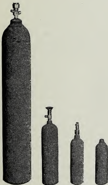
Figure 15.—Iron cylinders, for storing and shipping gases.
